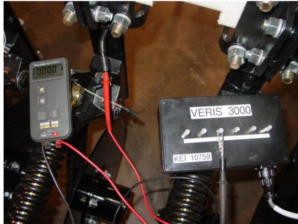
Figure 3.3 Testing cable at end of signal cable wiring harness
