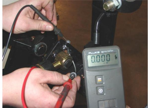
Figures 3.4 ab. a. Separating sure-seal connector b. Testing terminal connector wire
