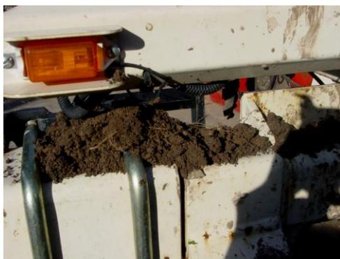
Figure 3.11 Wet soil buildup on toolbar may cause EC signal to short.
