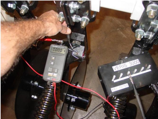
Figure 3.2 Testing cable at coulter electrode #3 terminal
