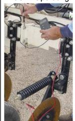
Connect one lead of an ohmmeter to each individual coulter electrode, and the other to a grounded fastener on the frame. Perform test on each coulter-electrode. Check ohms between all adjacent coulter-electrodes. If coulter electrodes are properly isolated, no readings will be obtained between coulters and frames or between adjacent coulters.
