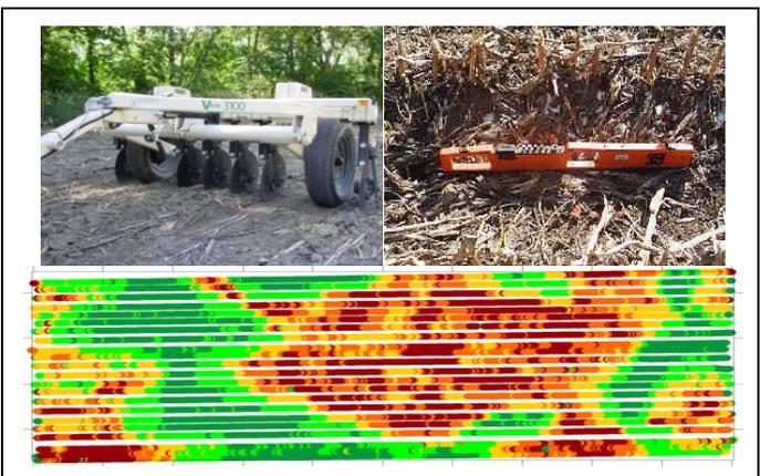
**Figure 1.** A Veris 3100 direct contact system with coulter-mounted electrodes requiring soil contact to measure soil EC (upper left) and a non-contact Geonics EM-38 sensor using electromagnetic induction to measure soil EC (upper right). A EC sensor coverage map acquired by Veris system for a field (lower image). (Veris images Courtesy of Veris Technologies and Geonics image courtesy of USDA-ARS)
