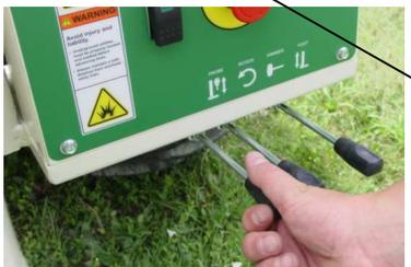
15. Pressing Probe button begins storing spectrum data and auxiliary data until probe is stopped or raised. Once insertion is initiated, do not stop or reverse unless problem has occurred or desired depth is achieved. Data recording stops when probe is raised. GPS and Log lights must be green for data to be recorded.
