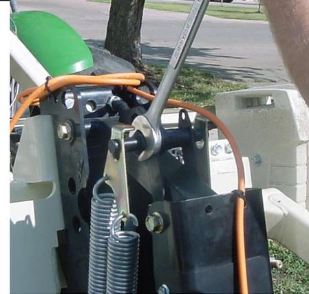
11. Adjust closing wheel pressure if needed to close slot. Pulling handle back increases pressure.
