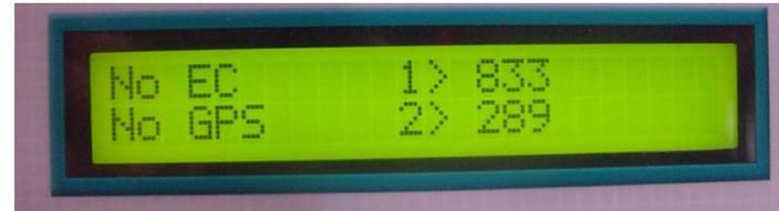
5. Clean sapphire window and install test reference under window. Click OM System check on Soilveiwier, or press 2 on Datalogger for OM System Check. Follow onscreen instructions. Reference values bellow.
