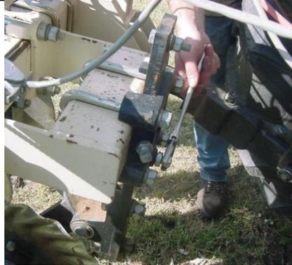
9. Adjust side depth wheels on optical row unit to allow deeper or shallower mapping. Move T-handle forward for deeper depth. Depth wheels should be snug, but freely moving, against the disks. See manual for adjustments.
